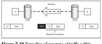
**Figure 7-10** Tunneling of one type of traffic within another, the basic premise of Virtual Private Networking
