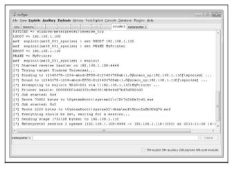
**Figure 4-4** Metasploit exploits the Microsoft Print Spooler Service Impersonation Vulnerability.
