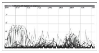
**Figure 9-11** Ubertooth Spectrum Analysis showing a large amount of activity in the lower part of the 2.4 GHz ISM band, most likely due to a high-speed 802.11 wireless network.
