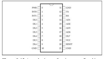
Figure 9-13 A mock pinout of a microcontroller chip
