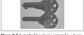
**Figure 9-2** A standard key (top) compared to a bump key (bottom). Notice the short, even-height teeth on the bump key.
