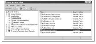
**Figure 4-1** Recommended audit settings for a secure server, as configured using Windows Server 2008's Security Policy snap-in
