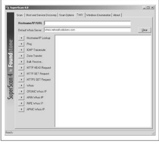
**Figure 2-6** The SuperScan tool provides a number of different assessment tools, many of which are discussed in other chapters.
