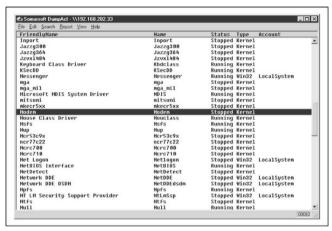
**Figure 3-6** DumpSec enumerates all services and drives running on a remote system.
