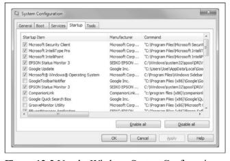
**Figure 12-2** Use the Windows System Configuration utility (Start | msconfig) to disable certain startup services.
