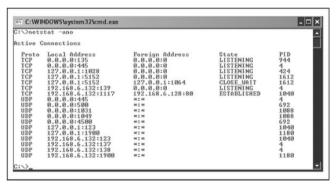
**Figure 6-7** Output of netstat command shows listening and transmitting processes.
