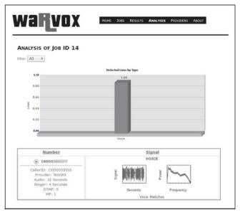
**Figure 7-2** The Analysis tab provides a summary of all of the lines dialed as well as individual call analysis that includes recorded audio; simply click the Play button.
