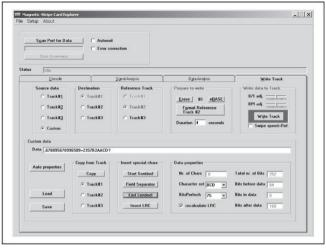
**Figure 9-5** Using Magnetic-Stripe Card Explorer to write custom data back to a card
