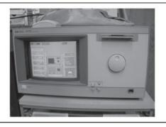
**Figure 9-15** A logic analyzer views signals traversing a bus.
