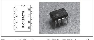
**Figure 9-12** The diagram of a PIC12F675 along with the photograph of an actual chip. Notice how the identifying marks on the actual chip may differ slightly from that of the diagram presented in the datasheet.
