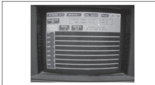
**Figure 9-17** A logic analyzer set to receive signals from the attached logic probes
