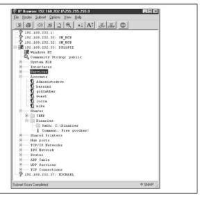
**Figure 3-9** SolarWinds' IP Network Browser expands information available on systems running SNMP agents when provided with the correct community string. The system shown here uses the default string "public".
