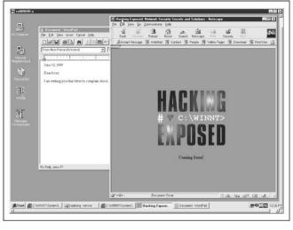
**Figure 4-9** WINVNC connected to a remote system. This is nearly equivalent to sitting at the remote computer.
