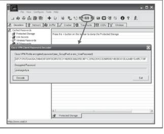
**Figure 7-12** Decoding the Cisco password 7 encoded passwords with Cain
