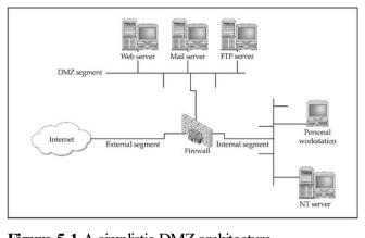
Figure 5-1 A simplistic DMZ architecture
