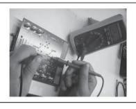
**Figure 9-14** Using a multimeter to create a component and bus map
