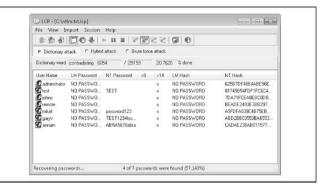
**Figure 4-6** LCP dictionary cracking NTLM passwords from a Windows Server 2008 system. Note that LM hashes are not stored in the default Server 2008 configuration.
