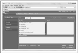
**Figure 3-1** The Nessus 4.4.1 web console. Notice that, at the time of this writing, it has 46,060 plug-ins, aka unique vulnerability checks! By the time you read this, it will have many more.
