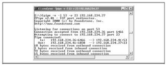
**Figure 4-10** The fpipe redirector running on a compromised host. Fpipe has been set to forward connections on port 53 to port 23 on 192.168.234.37 and is forwarding data here.
