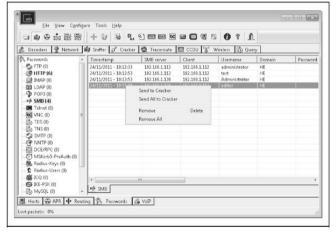
Figure 4-2 Cain sniffs NTLM authentication exchanges
