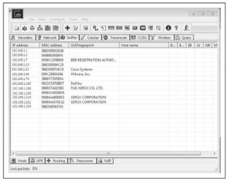
**Figure 2-1** Cain performs an ARP scan to identify live hosts on a local subnet.
