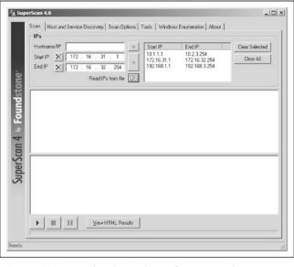
**Figure 2-3** By using SuperScan from Foundstone, you can discover hosts hidden behind traditional firewalls.
